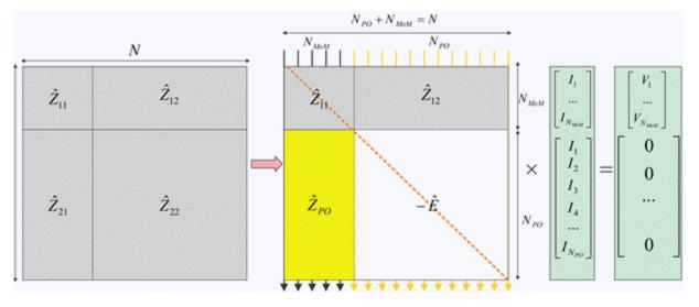
The figure shows the matrix interpretation of the hybrid MoM-PO solution and its comparison with plain MoM solution. The method assumes the antenna feeds gives the  $\vec{r}$
