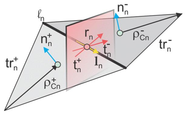
In the image, for two arbitrary triangular patches  $tr_n^+$  and  $tr_n^-$  having areas  $A_n^+$  and  $A_n^-$  and sharing a common edge  $l_n$  the basis functions has the form
