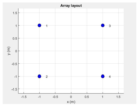
There are four ports in this array. The corresponding S-parameter matrix would be of size  $4 \ x \ 4:$
