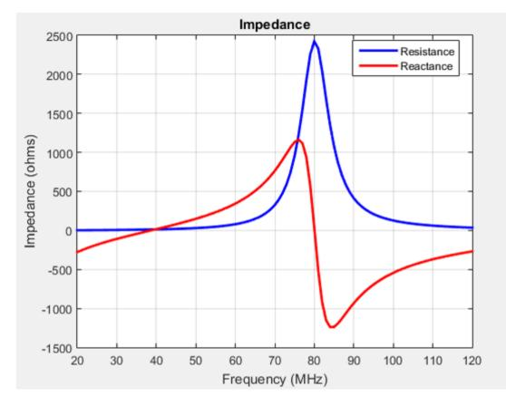
The resonance of the antenna further reduces to approximately 40 MHz.
