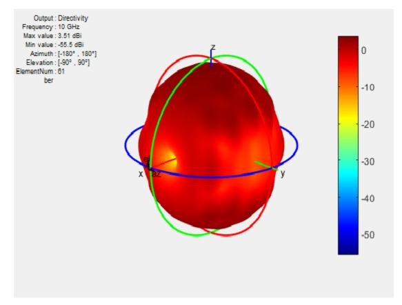
The figure shows the embedded element pattern of a center element in a  $11 \times 11$  array. You can also calculate the embedded element pattern as a magnitude of electric field.
