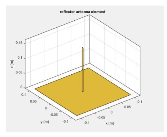
Rotating the reflector element rotates the entire structure by the specified angle. To rotate the complete antenna, use the Tilt property of the reflector object. For example, rotate the reflector by 90 degrees about the Y-axis. According to the right-hand rule, the reflector now lies in the Y-Z plane with the dipole.
