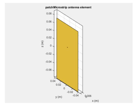
The patch lies behind the ground plane and is not visible. To make the patch visible change the TiltAxis property to [0 -1 0]. The Tilt property is still 90, but the axis of rotation is now the Y-axis. The negative number in the TiltAxis vector determines the direction of rotation about the Y-axis as per the right-hand rule.
