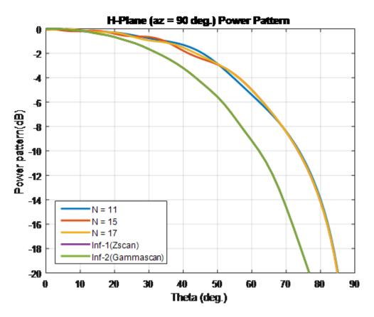
Case 2: Compare finite array and infinite array with unit cell of dimensions  $0.7\lambda \times 0.7\lambda$
