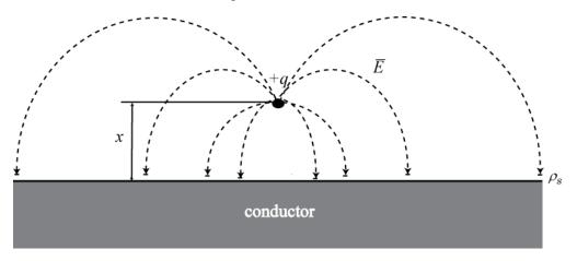
If you place a conducting object along this equipotential surface, then the field above the surface does not change.
