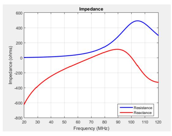
Use impedance to calculate the input impedance of any antennas in Antenna Toolbox.
