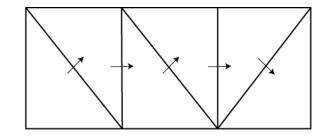
You formulate the problem by considering real and image basis functions. You can show the same problem using image theory or method of images. The interaction matrix is calculated using the interaction between real and image basis functions.
