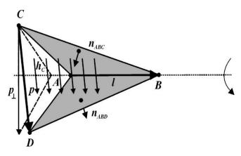
The figure shows an edge-based basis function. The vector variation is perpendicular to the base edge AB (or  $\overline{l}$ ). The vector of the edge CD (or  $\overline{p}$ ) defines the basis function. Within a tetrahedron, the basis function is a constant field given by
