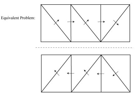
According to the method of images, the real and image electric currents are equal to each other in terms of magnitude. The parallel components are in opposite direction. The normal components are in the same direction.
