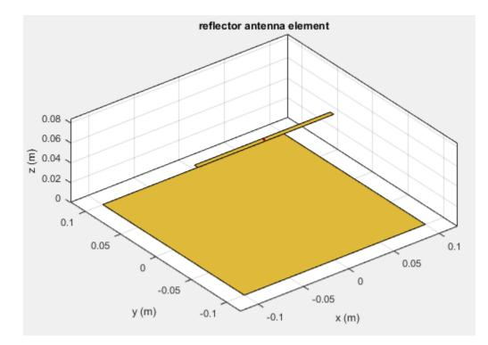
The dipole is the exciter element of the reflector. View its properties.
